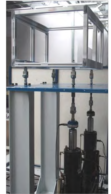
Durability test – multiaxial load
