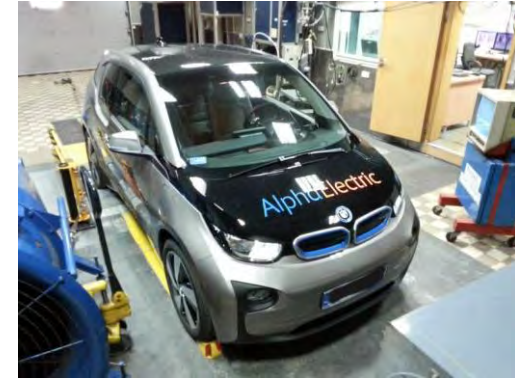
Large dimension climatic chamber Temp.: -45^{\circ}\text{C} - +75^{\circ}\text{C}
