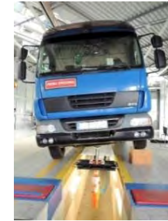
ABS and ASR testing
