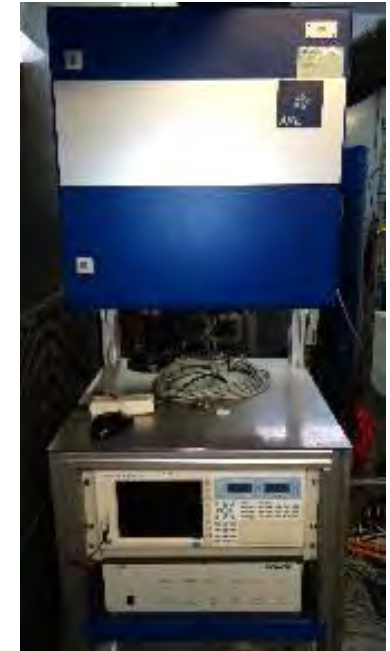
Power analyzer (Yokogawa unit)
