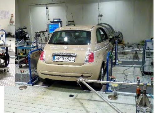
Large dimension climatic chamber Temp.: -45°C - + 75°C
