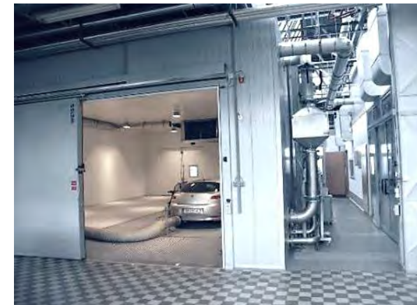
Climatic chamber (-35°C to +60°C) 14,3×10,1×4,3 m
