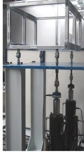
Durability test – multiaxial load
