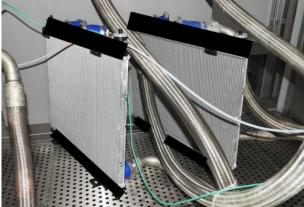
Internal erosion test
