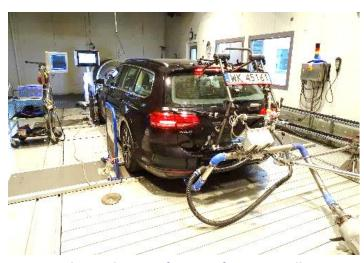
Chassis dyno verification of PEMS installation
