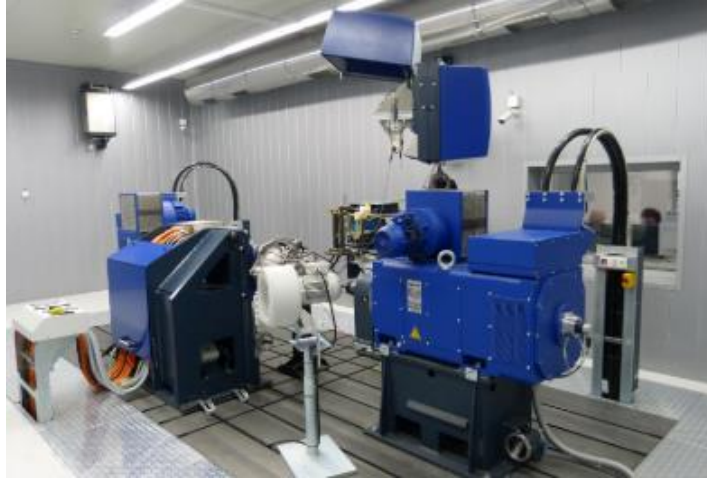
eDrive drivetrain testing with 250kW emulator
